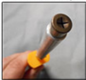
Place NW250 fastener onto Starlock Tool
