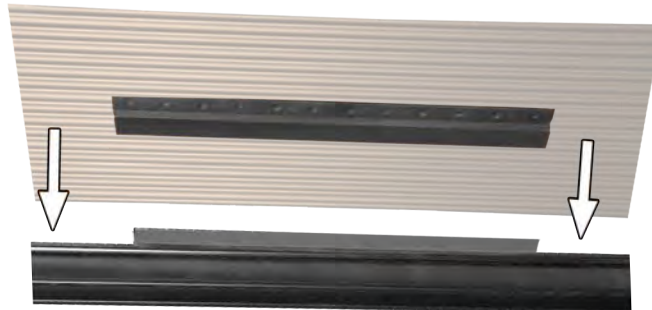
Picture of the back side of traverse track. Slide male portion of the Channel Lock located on the back of the fascia into the female portion of the Channel Lock located on the front side of the track. Then tighten them down using the set screws and wrench provided
